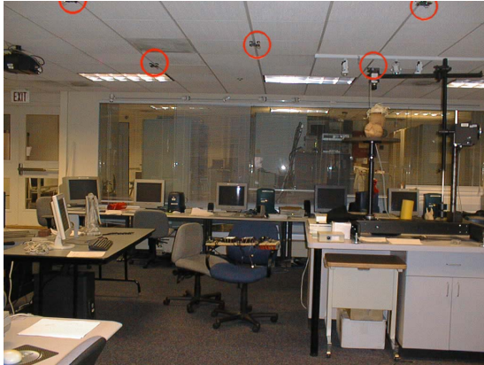
Figure 1.2: Example deployments of Cricket beacons. Multiple beacons may advertise the same space identifier if they are in the same space, but each beacon has a different position coordinate consistent with its location in space.
