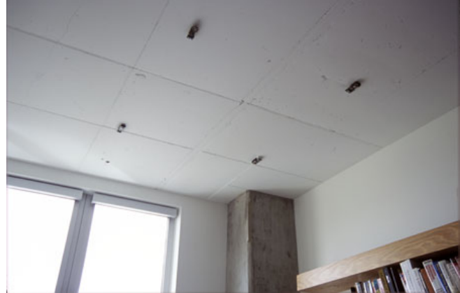
Figure 1.2: Example deployments of Cricket beacons. Multiple beacons may advertise the same space identifier if they are in the same space, but each beacon has a different position coordinate consistent with its location in space.
