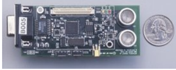
Figure 1.1: A Cricket hardware unit; this unit can function as either a beacon or a listener under software control, and can also be used in a more symmetric way as both listener and beacon.
